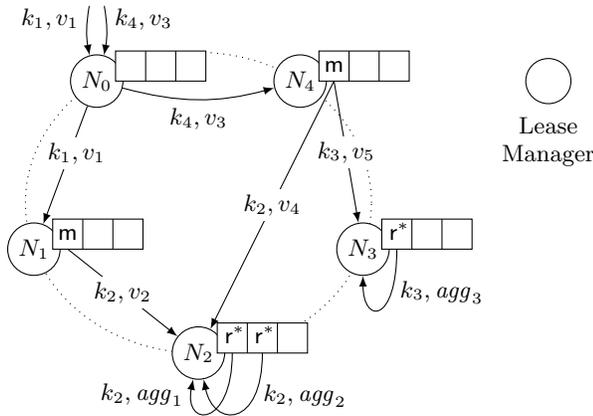
**Figure 3: Synchronization of reduce\* tasks (No replication shown)**
